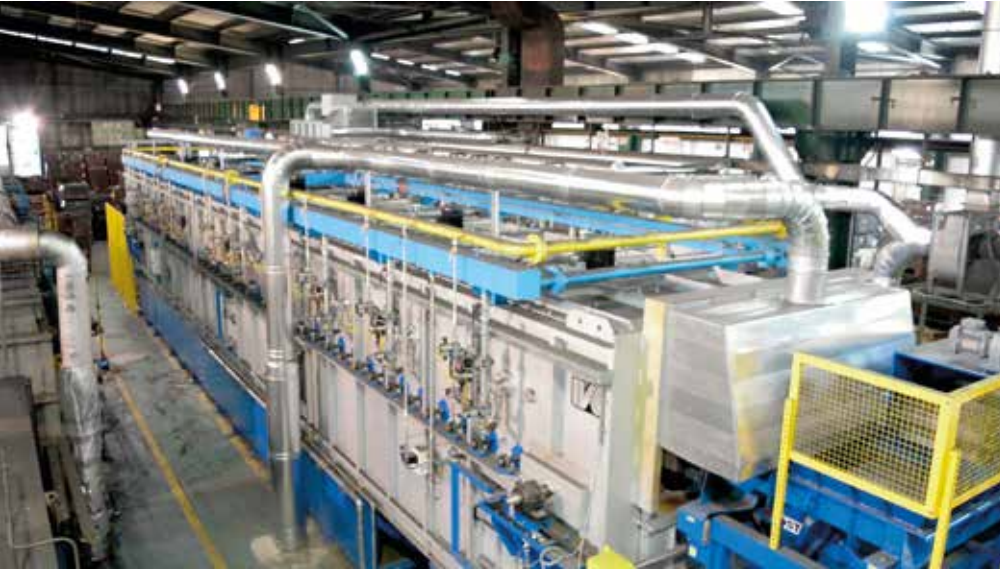
Example of continuous solution with casted belt for production up to 3000kg/h
